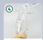
Add 50 ml of distilled, deionized or bottled water to the Whirl-Pak® filter bag.
