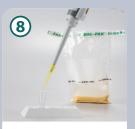
Transfer 100 µl of sample extract supernatant from the filter bag to the microcentrifuge tube (1:11 dilution).\*
